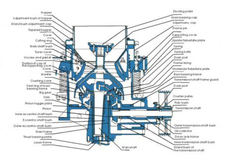
CS cone crushers are widely applied in cement making industry, building, sand making, metallurgical industry, etc. They are suitable for both metallic minerals and non-metallic minerals, such as iron ore, nonferrous metal ore, granite, limestone, quartzite, sandstone, pebble, etc.
