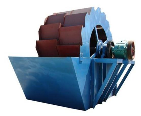
Sand washing machinery drives the impeller in the water groove to move like a circle transmitted by electric motor and decelerator, and then mixes, overturns, cleans and discharges the sand or slag pellets in the water groove.
